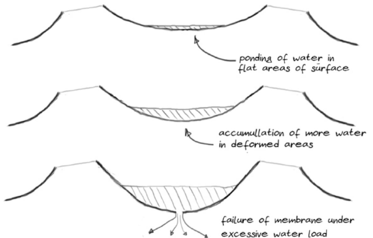
Figure 27. Sequence of water ponding on the area between two high-points: from rain-water accumulation to failure of the structure.
