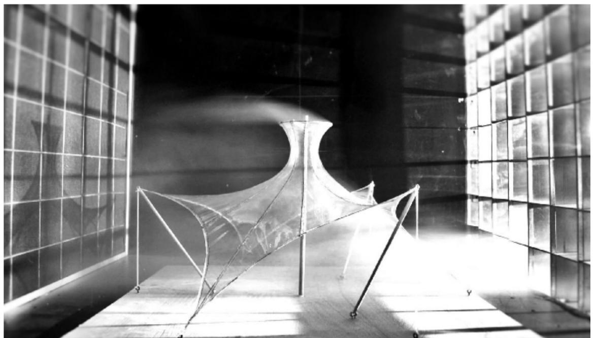
Figure 22. Diagram showing ventilation dynamics with the difference of pressure on an open conoidal high-point.
