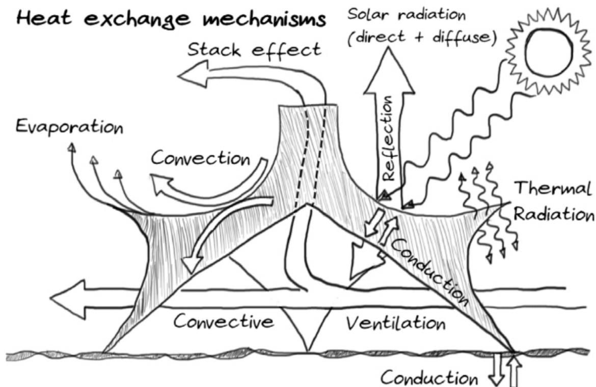
Figure 13. Heat exchange mechanisms on semi-open conoidal membrane structure.\*
