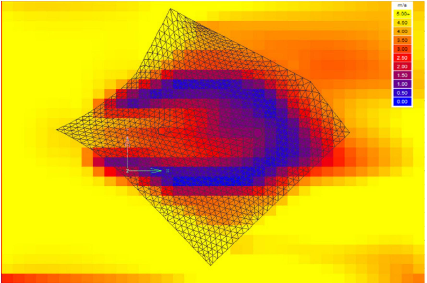
Figure 33. CFD airflow analysis showing air velocity membrane height in plan-view.
