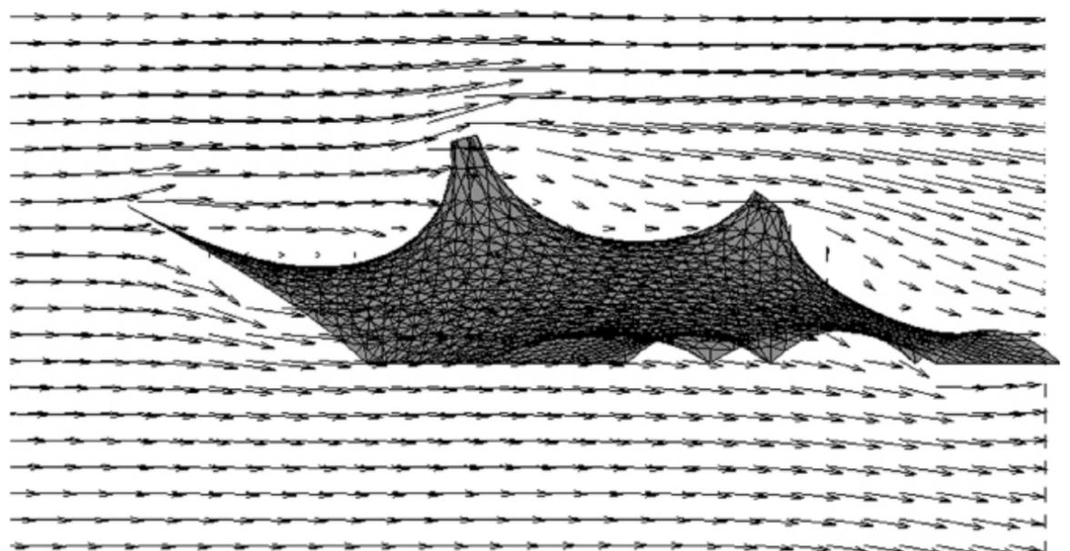
Figure 35. CFD airflow analysis flow vectors in section-view.
