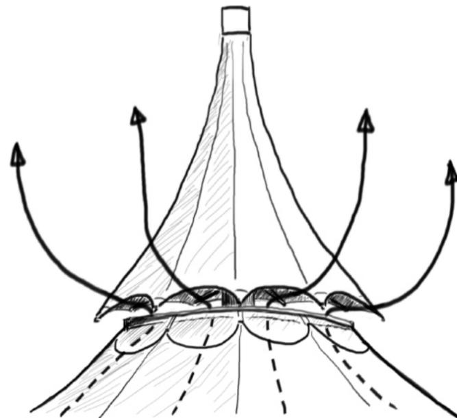
Figure 20. Ventilation strategy for double-skin-facades of a multi-storey building using modular saddle-shaped shading sails.
