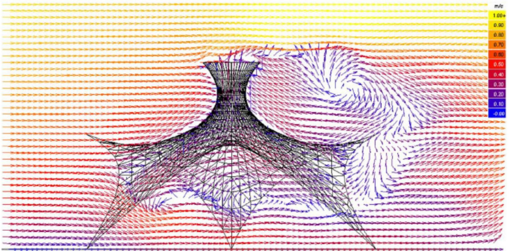
Figure 42. CFD analysis Air flow vectors and velocity (section view).
