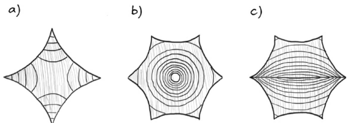
Figure 25. Isocurves of a sequence of height levels projected on different membrane geometries in plan-view: a) hyperbolic-paraboloid, b) conoid, c) arc.
