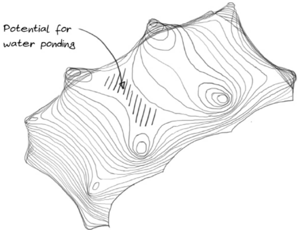
Figure 26. Analysis of drainage and potential areas for water ponding on a membrane structure with multiple high-points.
