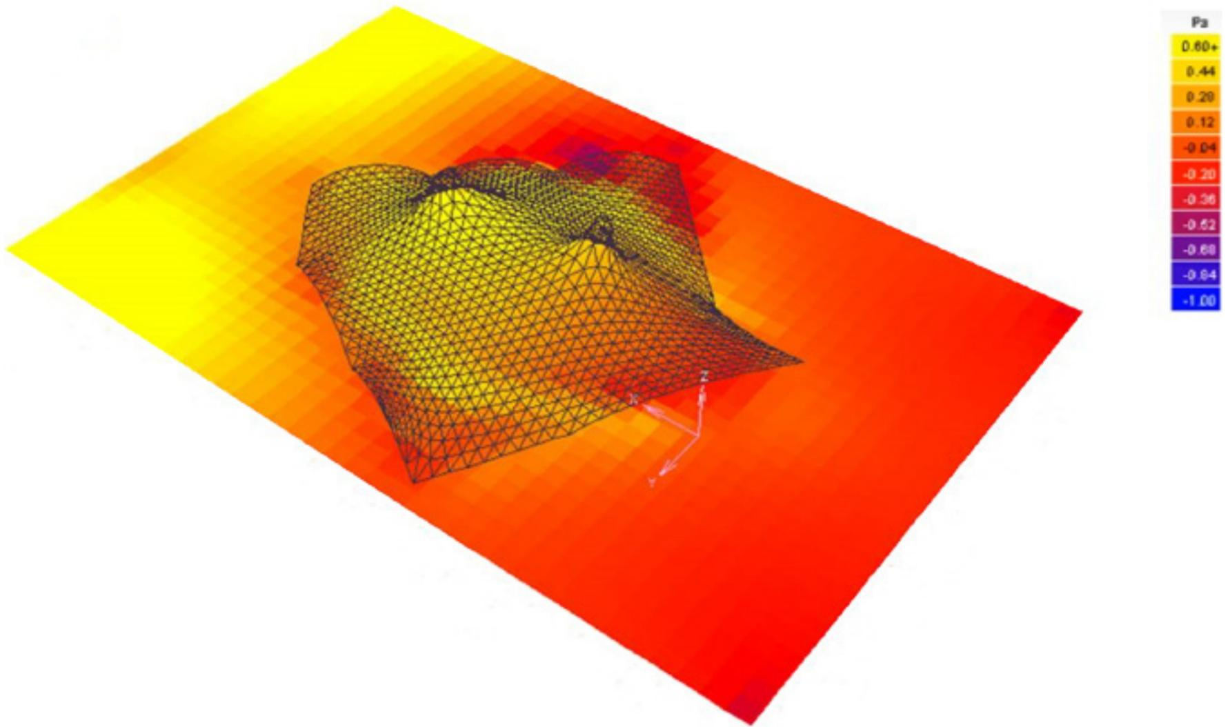
Figure 36. CFD airflow analysis showing air pressure at membrane height in perspective-view.
