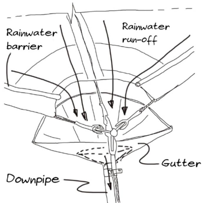
Figure 31. Drainage detail for membrane vertices with split gutters and flexible downpipes.
