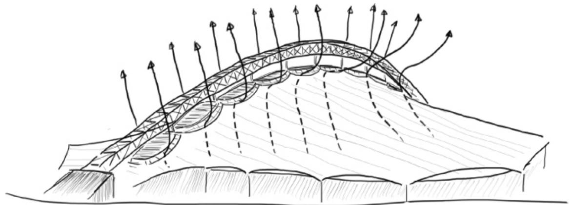
Figure 19. Ventilation detail for a high point on conoidal membrane structure.
