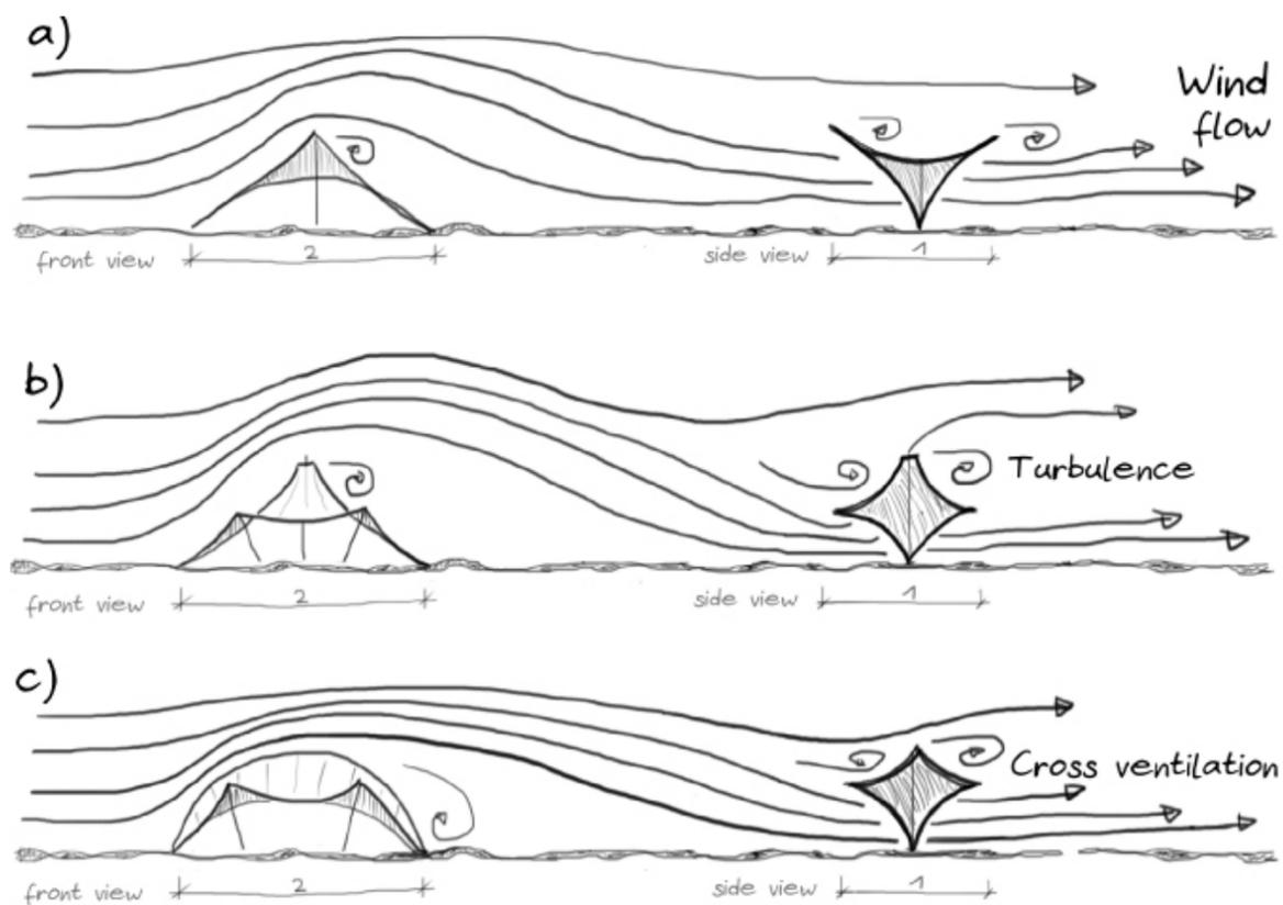
Figure 17. Improved ventilation with modified membrane structures: a) hyperbolic-paraboloid, b) conoid, c) arc.
