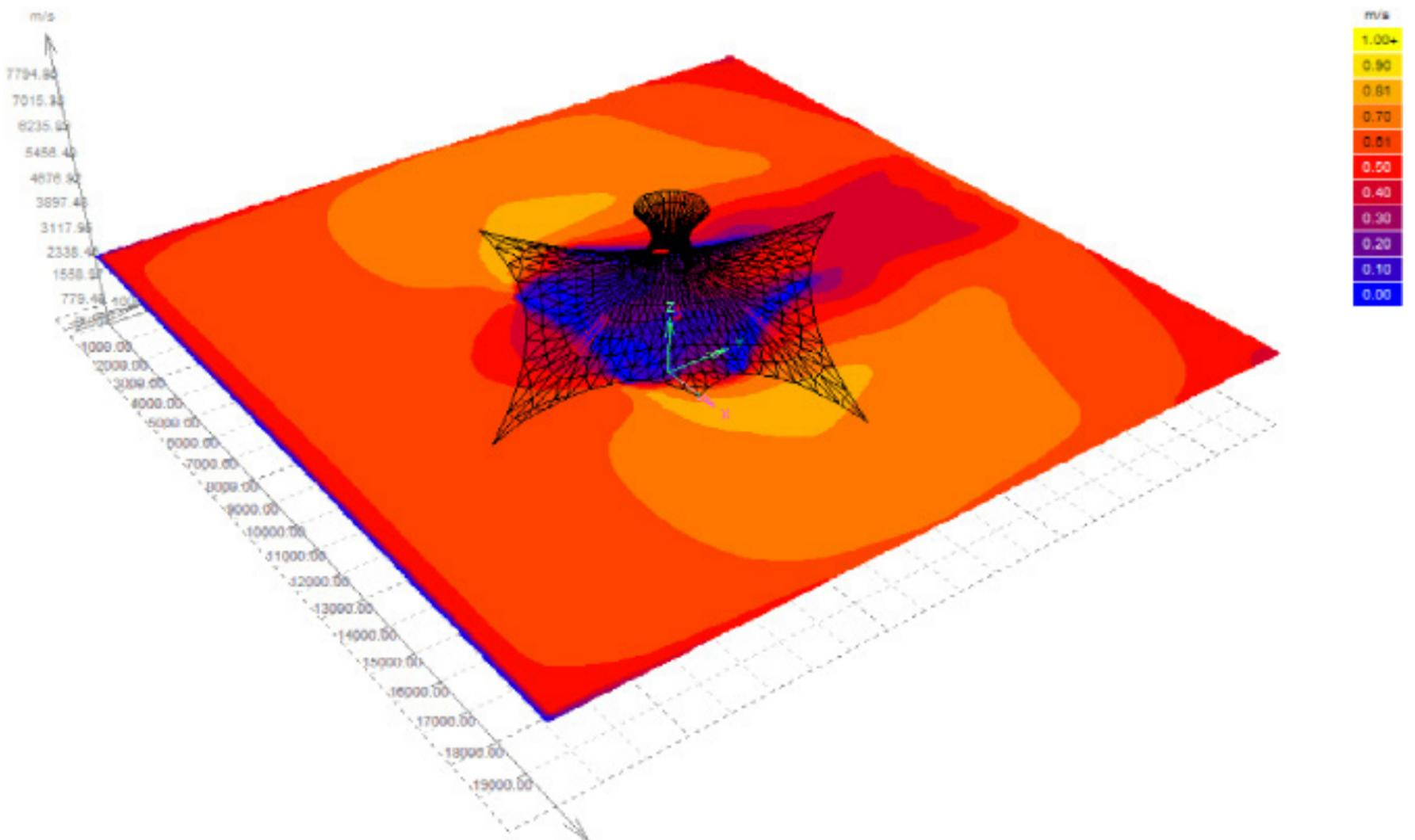
Figure 43. CFD análisis showing air velocity at membrane height (perspective view).
