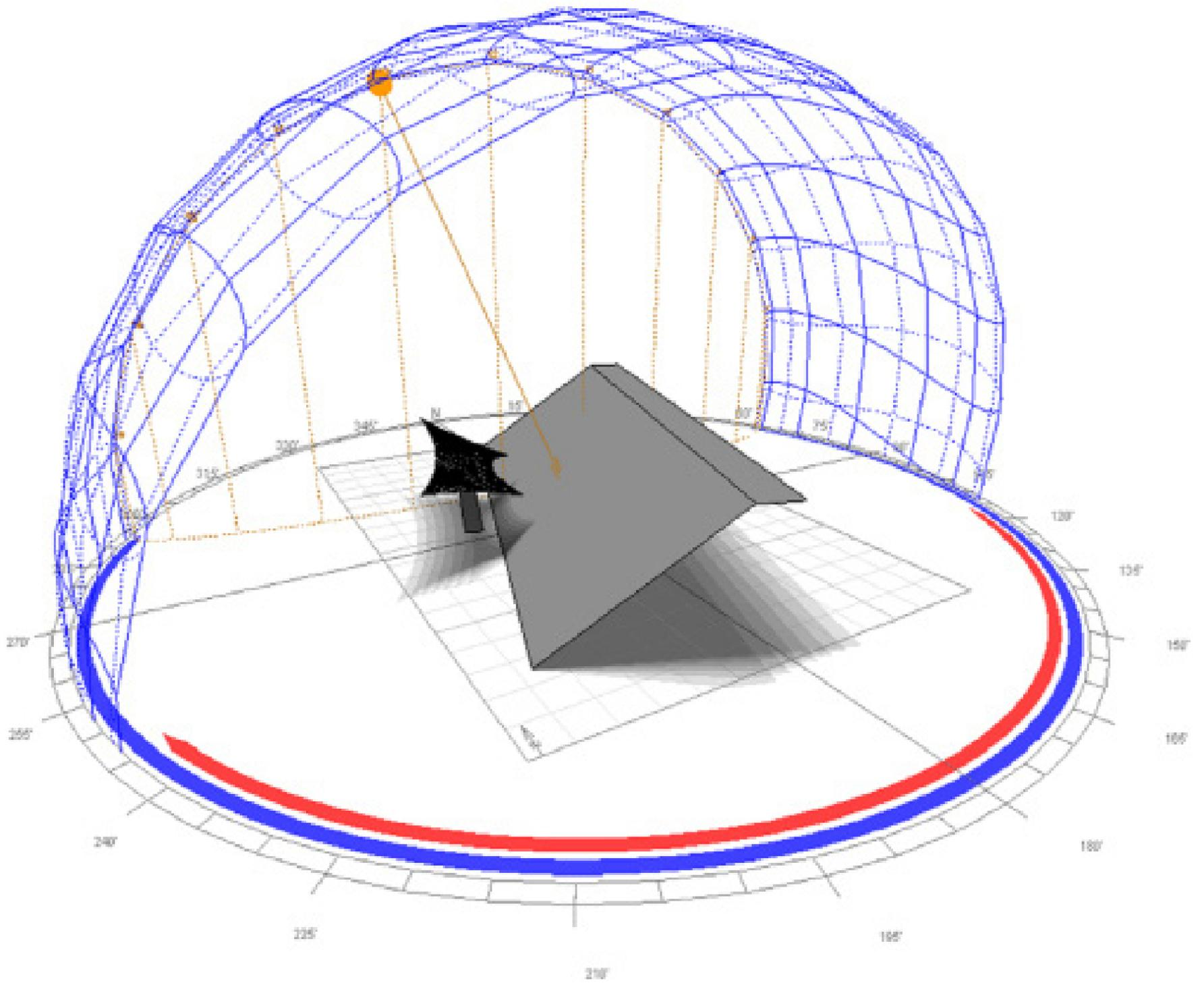
Figure 38. Three-dimensional solar sun path diagram with hourly shade projection. Source: (Image) elaborated by the authors.
